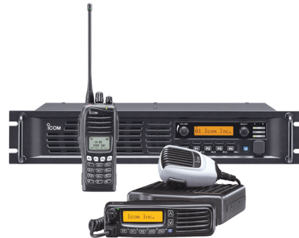
Pictured above: the FR5000 repeater. The board is installed in this repeater for trunking. Also shown the IC-F3161 and the IC-F5061.
